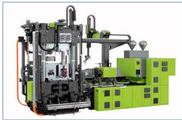
Fig. 5. Working in the direction of gravity offers benefits in many applications where preforms are used. The example shown in the figure is a system layout for an integrated multiple component process on a vertical injection molding machine (source: Engel)
