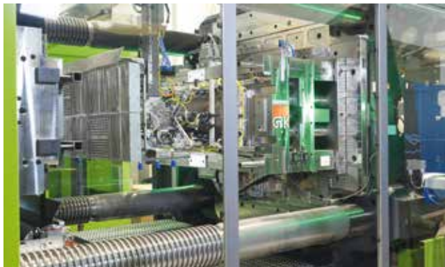
Fig. 3. The infrared heaters for heating up the film are integrated into the linear robot's grippers
