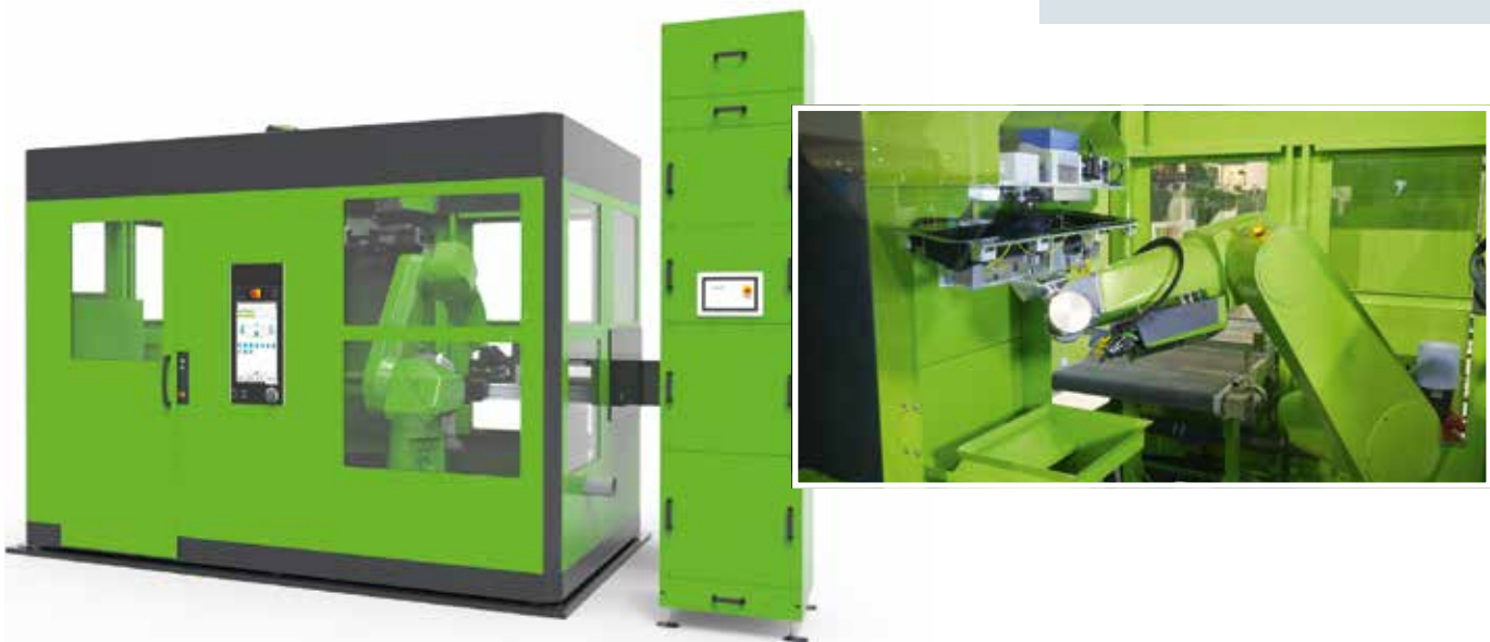
Fig. 5. For the DecoJect process, the easiCell automation cell (left) integrates a multi-axis robot and the laser station for trimming the demonstrator. The robot moves the component contour along the laser (right) and then places the ready-to-fit component on the conveyor belt (© Engel)
