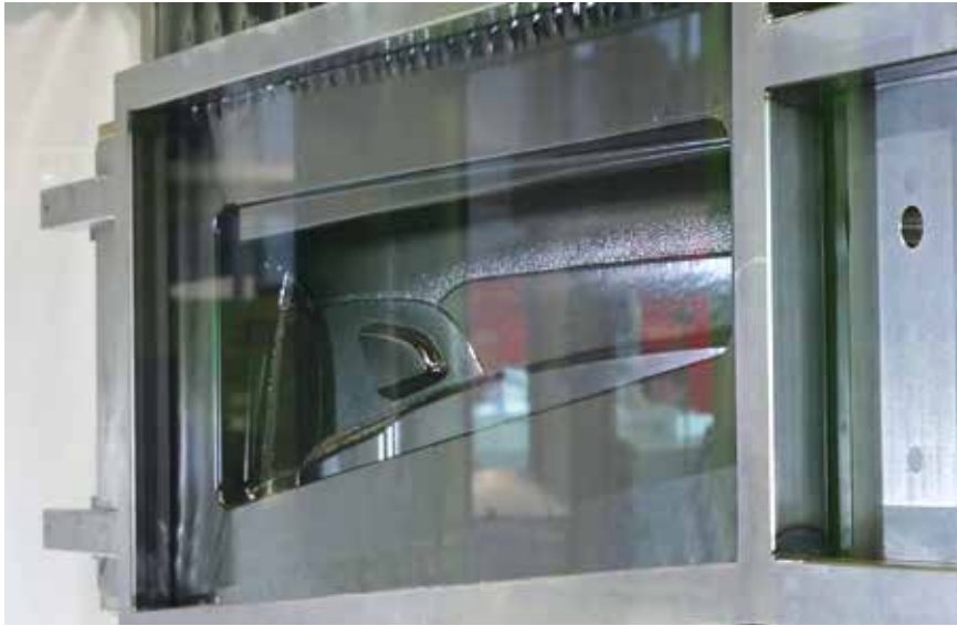
Fig. 4. The compression process starts during heating up by drawing the film (here: black) into the IMG mold (© Engel)
